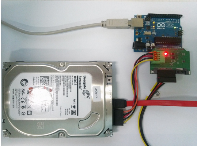
Fig. 1. Implemented power measurement device
